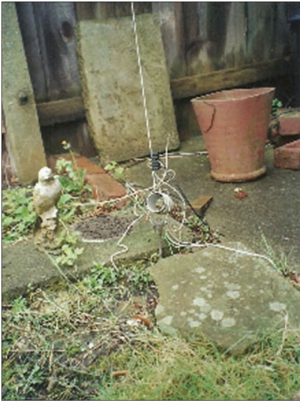
Fig. 2: View of the shunt coil, coaxial cable feed and earthing rods. The coil consists of seven turns of antenna wire wound on a 50.8mm (2in) former. Some form of weather protection will probably be needed.
