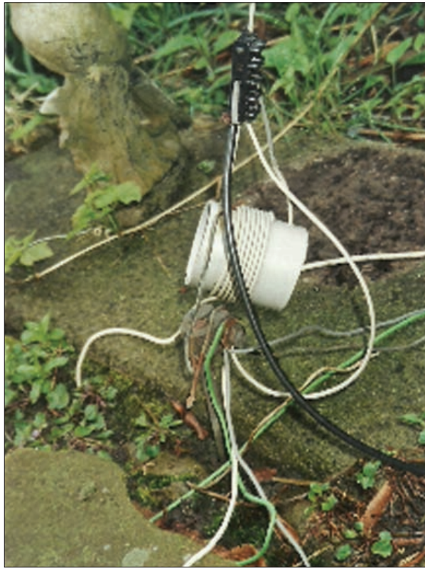
Fig. 3: Close-up view of the shunt coil. The coaxial cable from the transmitter is connected across the shunt coil - inner to the end out to the loading coil and top. The braid connects to the earthy side, going to the ground spikes and radials.
